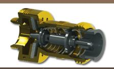
The patented NIDEL® Model 50HF high flow double check backflow preventer is standard equipment on specified Roof Hydrant models. It is intended for irrigation and outdoor watering and is designed to protect hose connections from backflow contamination in freezing and non-freezing conditions.
